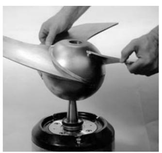
Lift the propeller onto the shaft.
