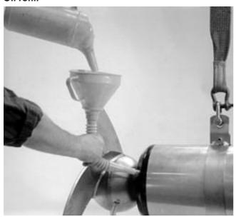
Fill up with new oil in the oil filling hole, the mixer should be in a horizontal position. Always replace the O-rings (24) of the oil hole screws. Put the screws back and tighten them. Tightening torque 10—20 Nm (7.4—15 ft lb).
