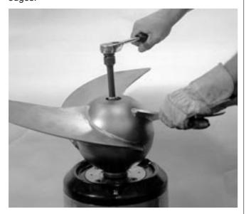
Remove the protective cover and the O-ring.
