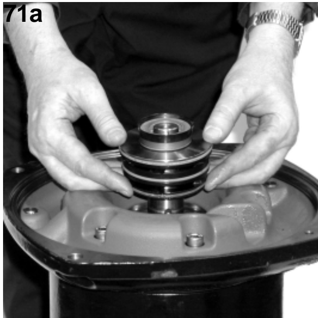
71a. Grease the shaft. Fit a new mechanical seal unit (oiled). N.B. Check that the drive pin engages in the drive groove in the shaft. (Picture shows version without cooling jacket)
