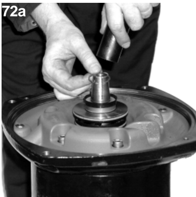
72a. Fit the circlip (picture shows version without cooling jacket).
