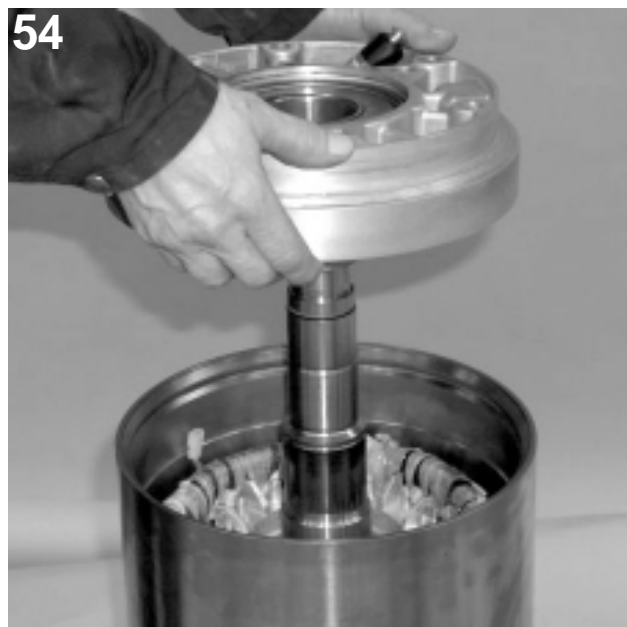
54. Oil the rotor shaft. Place the bearing holder on the shaft.
