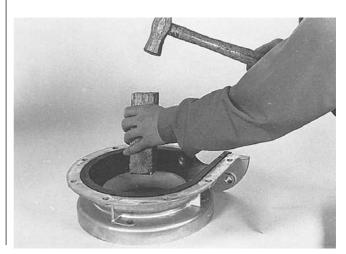
Remove the rubber cap (95). Lock the impeller (31) using a pliers, remove the impeller nut (89) and the lock washer (66).
