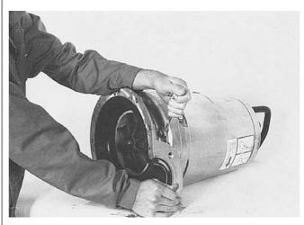
The rubber parts (46) can be prized off with a screw-driver.
