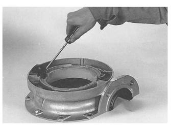
The upper rubber lining (18) and the wear ring (45) can now be replaced.
