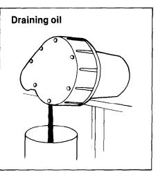
Refill the oil casing with 1/10 litre (1/6 pint) of SAE 10W-30 oil.
