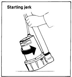
the instant of starting. If it jerks the other way, switch two phases in the motor control. Running the pump in the wrong direction of rotation means reduced capacity and strains the motor.
