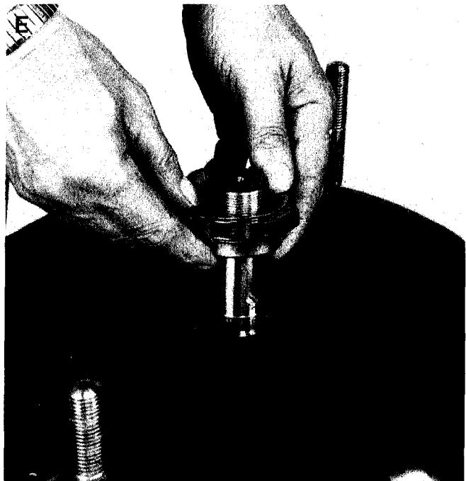
Remove the sleeve (135) together with the seal ring (133). Press the sleeve out of the seal ring.
