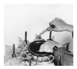
Turn over the pump and fit the spring assemblies consisting of spacer sleeves, rubber bushes and coil springs.
