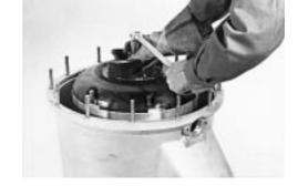
Fit a screw, 81 40 21 (M 16) into the threaded washer located under the impeller screw.
