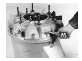
If the diffuser is difficult to lift off, put back the lower diffuser and secure it with three nuts. Pull off the diffuser with puller 84 13 60.
