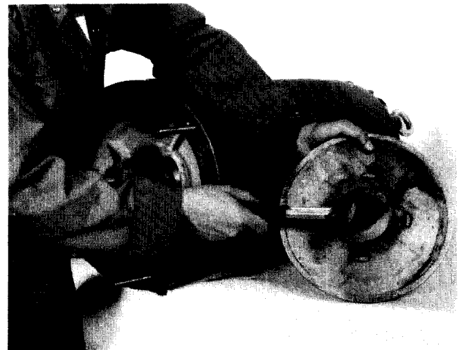
After the four screws (5) have been removed the washer (106) can be knocked out.
