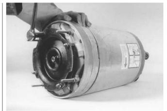
Remove the nuts (15) and the washers (21) on the diffuser ring (76). Pull off the diffuser ring.
