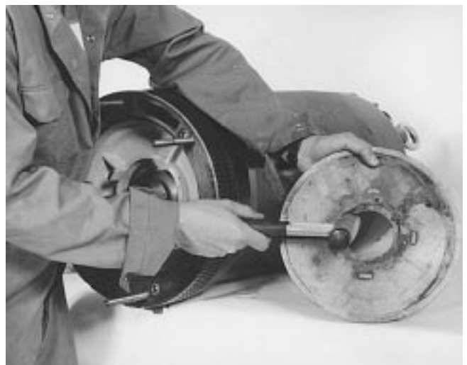
After the four screws (5) have been removed the washer (106) can be knocked out.
