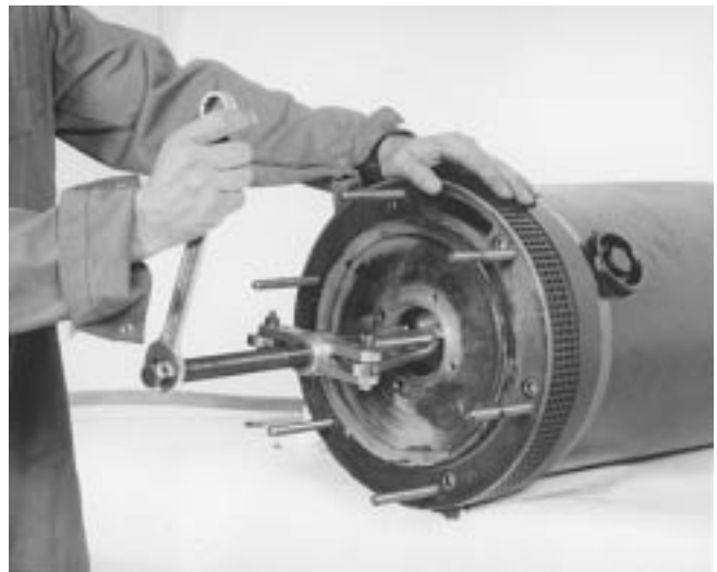
Pull of the diffuser disc (113) with a puller.
