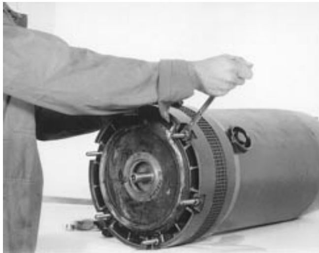
Remove the nuts (13) from the stud (89).
