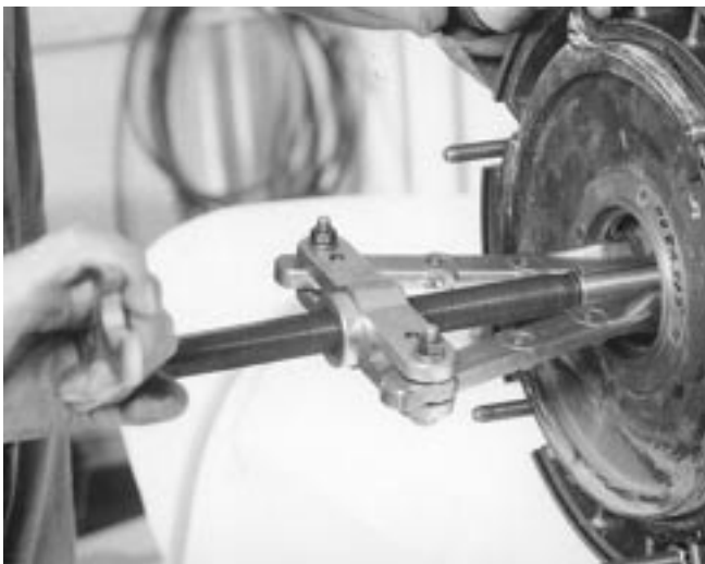
Pull of the upper diffuser (112) with puller.
